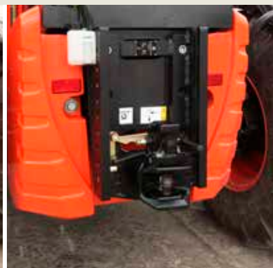
Rotating tow hitch with height adjustment
